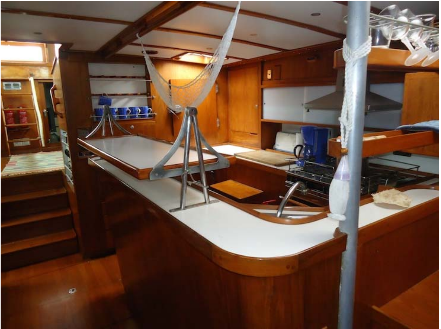
The spacious galley features a unique gimballed serving area for full plates and glassware while heeling underway.
